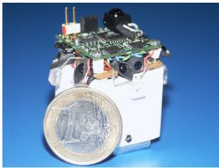
Figure 3: The prototype of the "Jasmine" microrobot.
